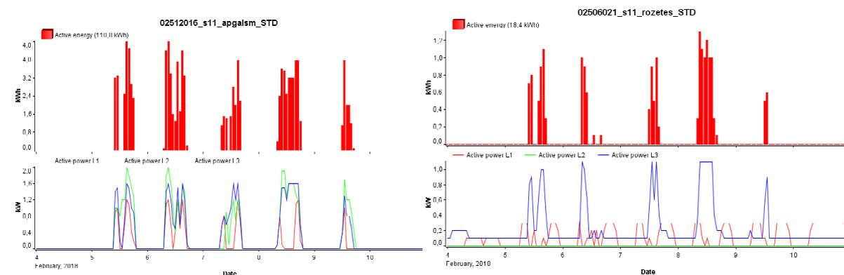
Fig. 4. **Room level auditorium electrical energy consumption data:** auditorium lighting (left), power supply sockets for presentation equipment (right)
