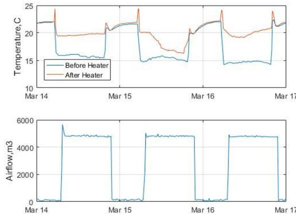
Fig. 5. Experiment results in PN6 zone level using 6 kW heater
