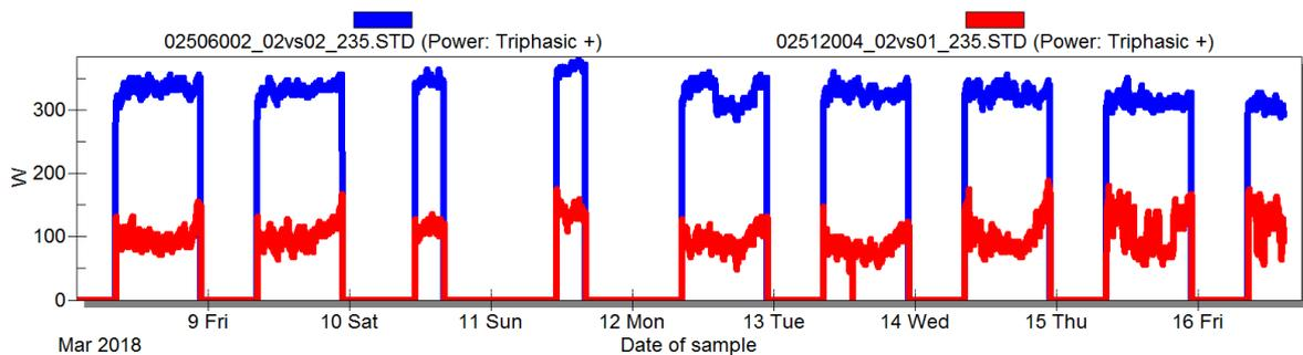
Fig. 6. Power consumption measurements (red – PN1; blue – PN2)
